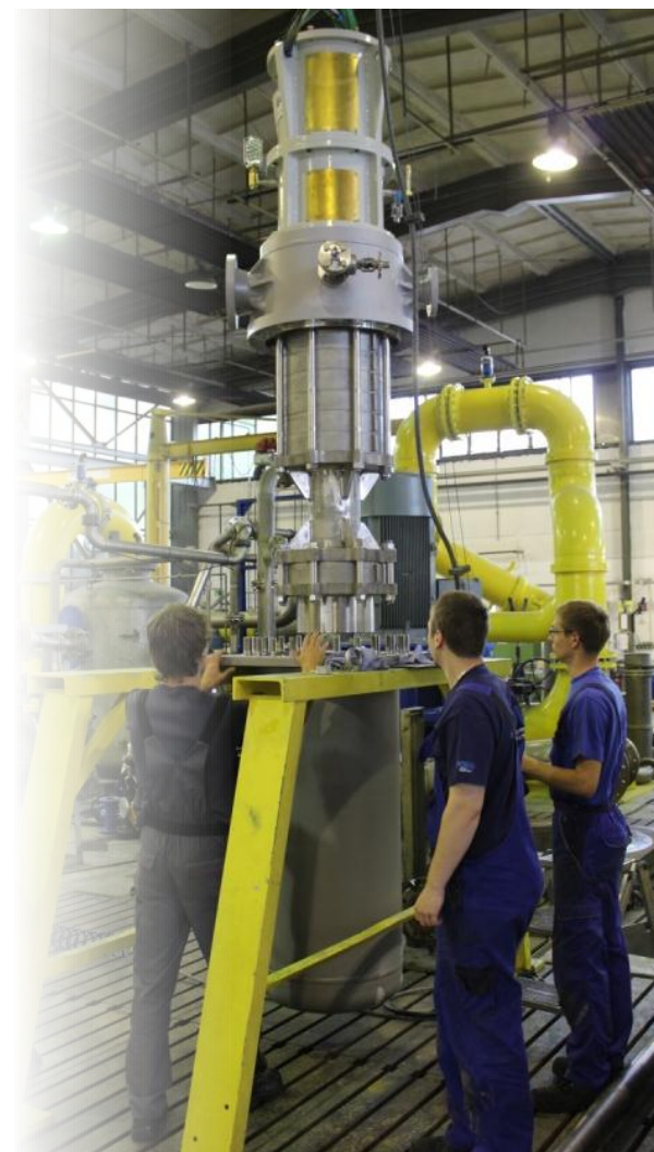
Vertical API 610 pump at the testing bed
